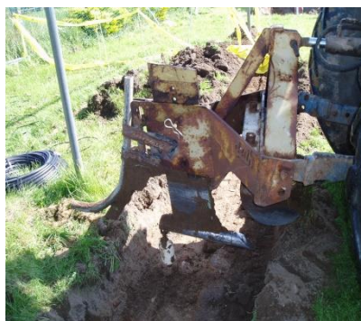
Mole plough attached to farm tractor
